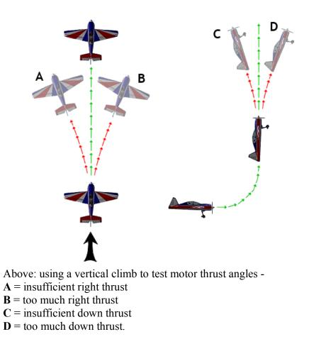
Another simpler way to test the down thrust is to fly the straight and level pass at about 1/2 power, then quickly apply full power. If the plane pitches up wildly then you need to increase down thrust. If the plane suddenly pitches downwards when you apply the power, the down thrust is too much. Ideally you are looking for nothing more than an increase in speed and a slight gain in altitude when you increase power, this gain being a result of the increase in lift as the airspeed increases.
