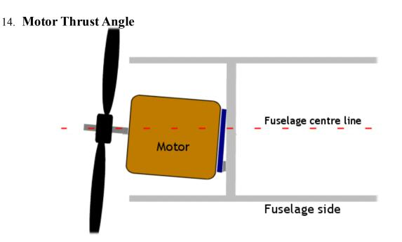
Thrust angles are factored in to an rc airplane's design where necessary. The two common types of thrust angles are **right thrust** whereby the motor is angled slightly to the right, when viewed from above, and **down thrust** whereby the motor is angled downwards slightly.
