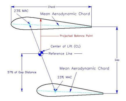
Once you have the MAC for both wings and the CG balance point as a percentage of the MAC, connect the two CG positions with a line. Measure up between the wing Gap distance and place your center of lift (CL) at the 57% reference line. Project this location up and balance your biplane at this postion (see red lines). A CG forward of the CL makes the model more stable, Placing it aft of the CL makes model less stable. Simple Method to Find CG:
