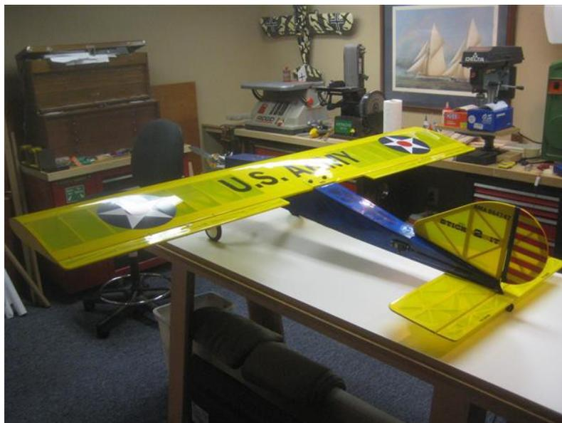
*After covering, reinstall all the components and glue in the aileron CA hinges.*
