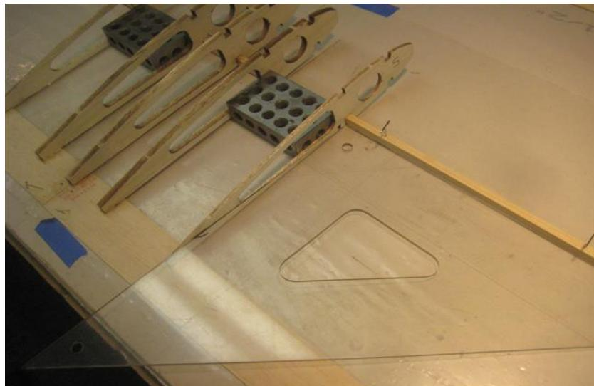
*\*Place two # 3 ribs each side of the wing center line spaced 3" from the previous installed # 2 rib and from each other, with their bottom notch over the bottom main spar and the rear end of the rib on the rear sheeting. Make sure the ribs are 90 degrees to the work surface and the main spar. There should be a no gap between the bottom of the ribs and the work surface. Glue in place.*
