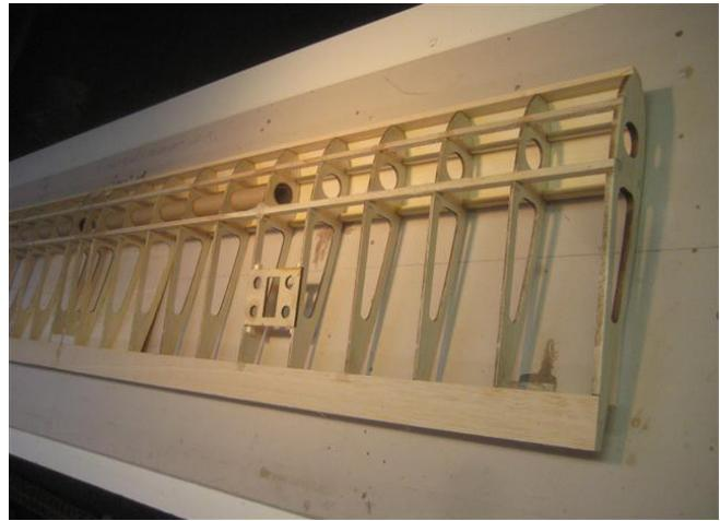
*\*Cut, fit and glue in place 1/16" balsa webbing against the back of the spars from the #2 ribs left side to the #2 ribs right side. Make sure the webs are flush to or below the bottom edge surface of the ribs.*
