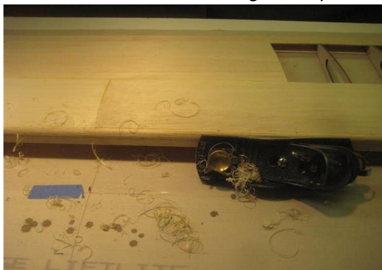
*\*The end caps should be positioned on the out board surface of the last rib and glued in place. The periphery of the end cap should be sanded to match the wing surface and a small radius applied to the end cap.*
