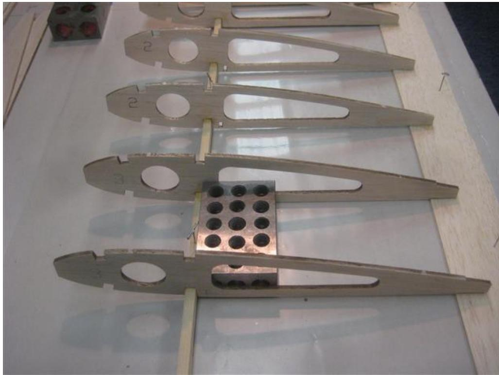
\*Place one # 4 rib each side of the wing center line spaced 3" from the previous installed # 3 rib, with its bottom notch over the bottom main spar and the rear end of the rib on the rear sheeting. Make sure the rib is 90 degrees to the work surface and the main spar. There should be a no gap (except for the wing servo tray notch) between the bottom of the rib and the work surface. Glue in place.
