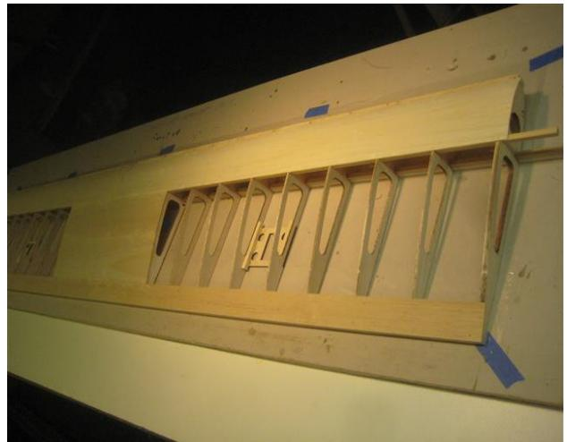
*\*Trim off all the existing spars, stringers, and sheeting that may be beyond the outside surface of the last rib. Clean up any glue joints that may have excess glue that will interfere with the construction of the bottom side of the wing.*
