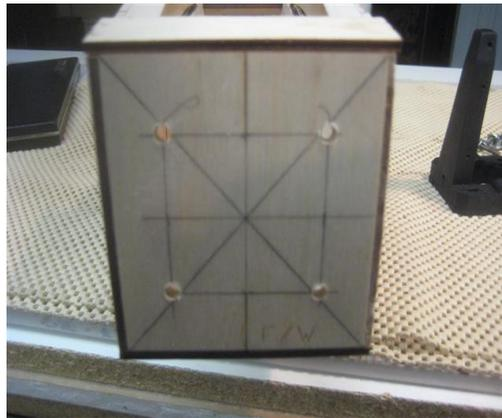
*\*Position and glue in place the bottom I/s reinf. Front.*
